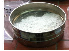
f- Waste Sample After Screen Process.
